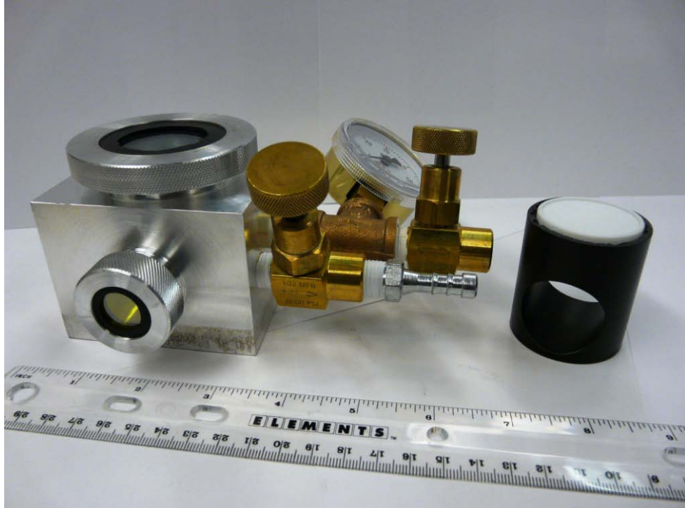
Figure 3.02. A photograph of photoreactor, cylindrical block made of Delrin and sample dish made of Teflon
